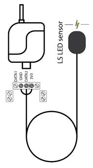
10.1. Measuring electric energy with external optical sensors LS
